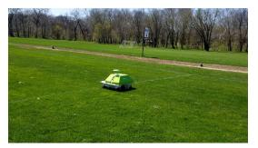
Optimus is the name of the league's GPS field lining robot and the little green guy is a life saver. What used to take three hours, now can be completed in a little more than 40 minutes. With the aid of a base station, we simply load our field template into a hand-held tablet and press play.
